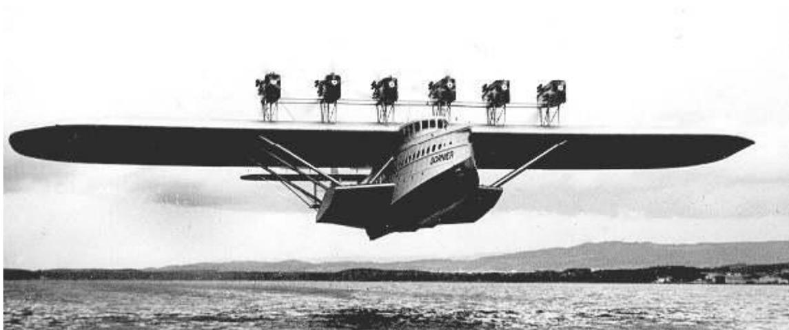
**Dornier Do-X, after having been modified, takes off with the full power of its 12 Curtiss engines**
