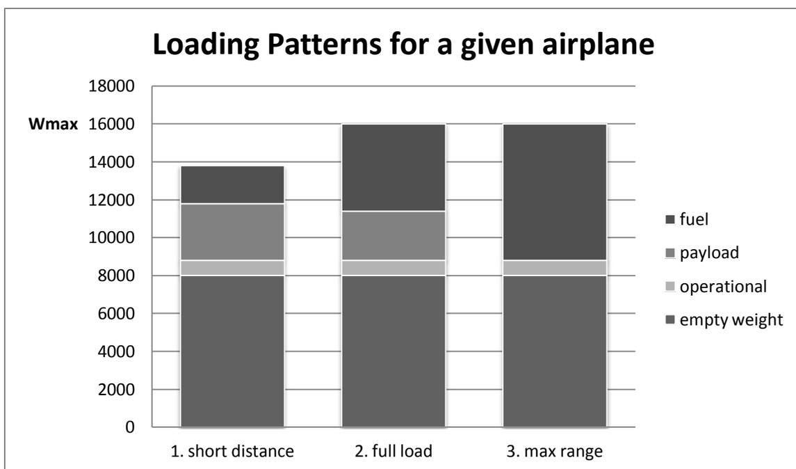
Fig.3 Loading Patterns (example)
