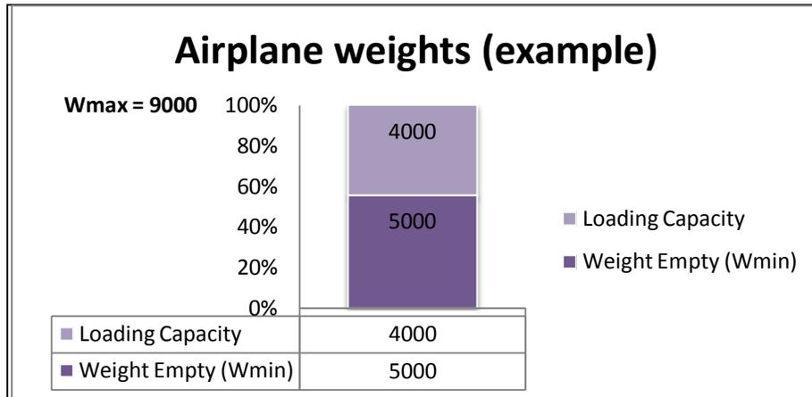
Fig.1 Definition of Weights and Loading Capacity
